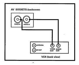
Connect the VIDEO in and AUDIO in sockets of the TV to the VIDEO out and AUDIO out sockets of the VCR for playback programmes. (Applicable to sets with AV mode only)
